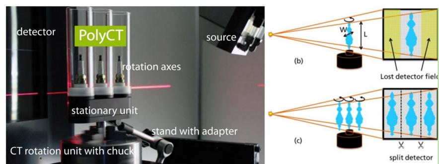
Figure 1 Principle of Poly CT Add-On
