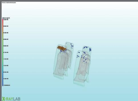
3D examination (CT) with voids analysis. It is possible to determine the defect volume as well as the volume of the object. Each individual inclusion can be evaluated separately in volume, diameter and geometry.
